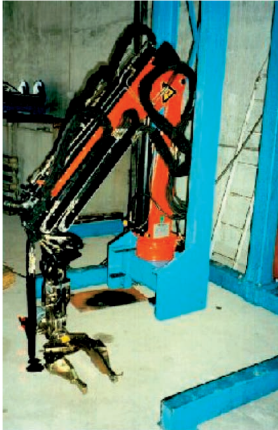
FIG. II-3. Small crane inside a cell.
