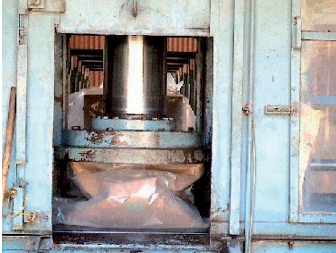
FIG. V-4. HEPA filter compaction stage.
