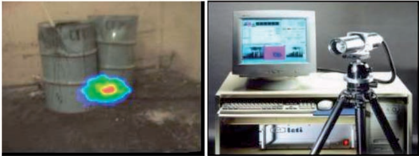
Localization of contamination in waste drums
